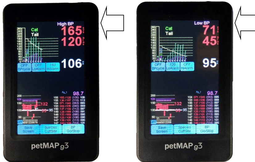
High BP Alarm
