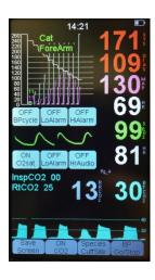
4) When the warm-up is complete, the bottom portion of the petMAP display will look like this if Pg\_4 is selected, displaying the capnograph, ETCO2 value and RRCO2 (Respiration Rate from CO2). InspCO2 (Inspired CO2) and RtCO2 (Realtime CO2) are also displayed.
