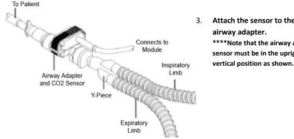
Attach the sensor to the airway adapter. \*\*\*\*Note that the airway and sensor must be in the upright
