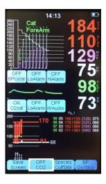
2) Turn CO2 ON by pressing the highlighted CO2 ON/OFF button on the bottom of the petMAP display.
