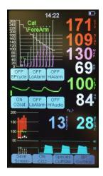
6) When monitoring is complete, turn CO2 OFF by touching the ON CO2 button.
