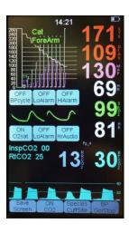
4) When the warm-up is complete, the petMAP+II display will look like this if Pg\_4 is selected, displaying the capnograph, ETCO2 value and RRCO2 (Respiration Rate from CO2). InspCO2 (Inspired CO2) and RtCO2 (Realtime CO2) are also displayed.
