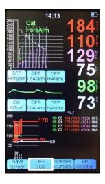
2) Turn CO2 ON by pressing the highlighted CO2 ON/OFF button on the petMAP+II.
